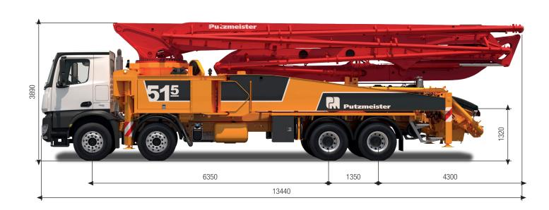
Note: Serial version. Dimensions and weights depend on truck, pump model and equipment. Dimensions in mm, MB Arocs 4144 as example. For illustration only.
