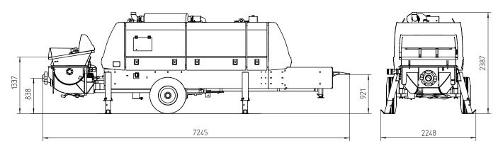
Note: Standard version BSA 2110 HP D. Dimensions and weights depend on equipment. Subject to technical modifications and errors.
